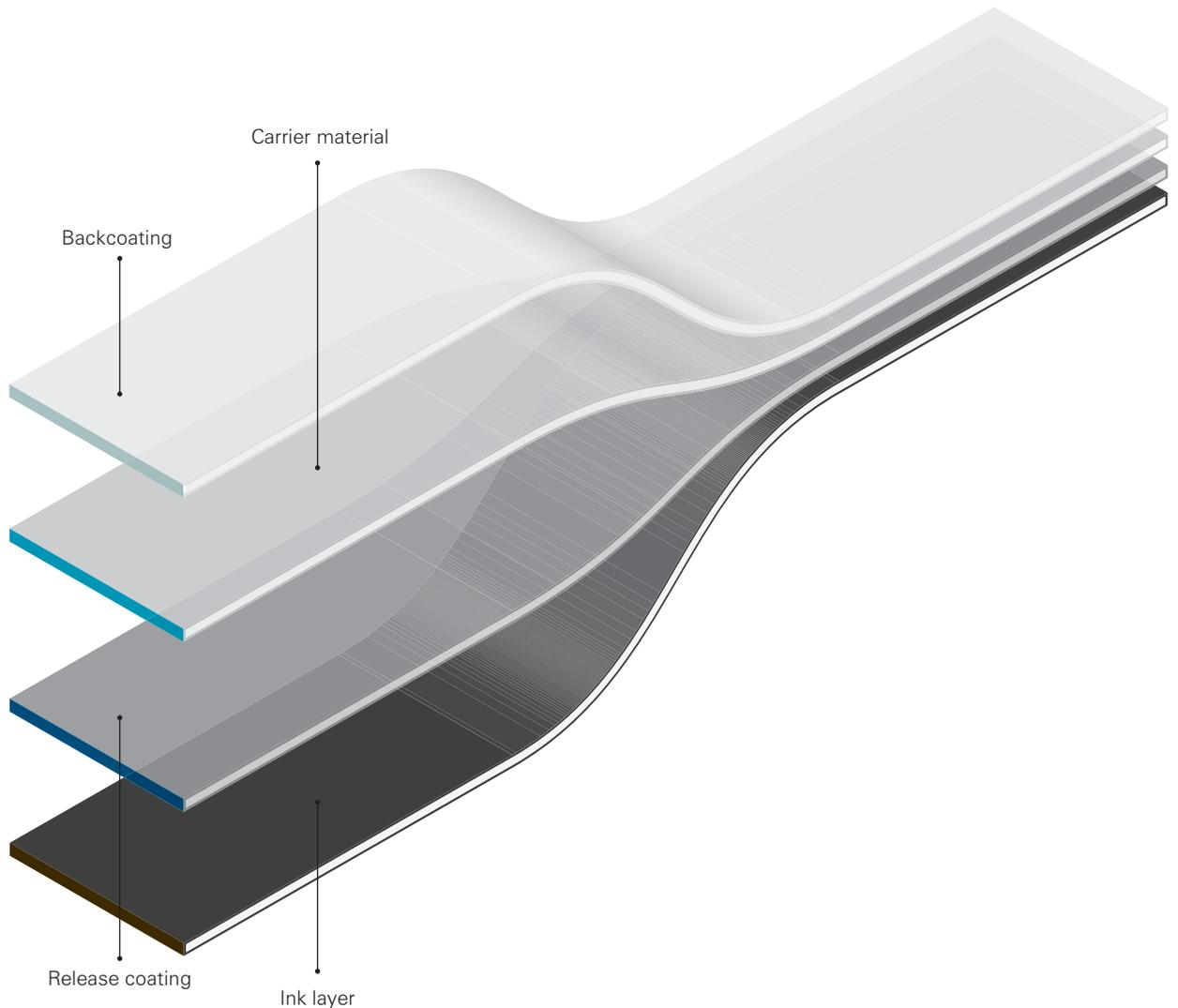
The composition of a ribbon is integral to how the ribbon performs. Zebra considers each element of the ribbon to ensure optimum performance is achieved in Zebra printers.
