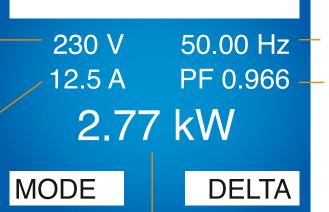
Power measurement (kW) The effective power drawn by the consumers, taking the phase angle into account. Power consumption of the con-
