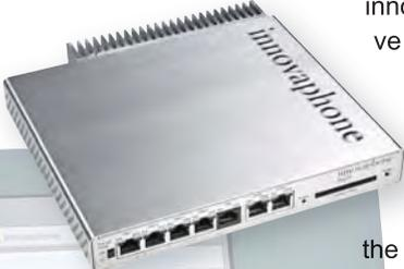
innovaphone **VoIP gateways** serve as the interface to other networks, at the same time forming the hardware platform for the innovaphone PBX. The innovaphone PBX software is pre-installed on the devices and can be activated easily with the appropriate license key. The various gateways have different types and numbers of interfaces which can also be activated using licenses. Any number of gateways can work together as a network for larger installations across multiple locations.
