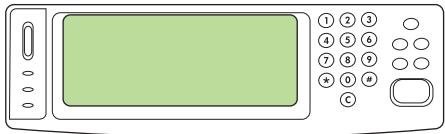
**EN** • To reset the maintenance kit page count for the HP LaserJet 9040mfp/9050mfp. Press the power button to turn the MFP on. When the memory count starts, press and hold the **6** button. When the three LEDs are on, release the **6** button. **Select Language** appears on the screen. Press and hold the **3** button until **New Maintenance Kit** appears on the screen. Press and release the **6** button again.
