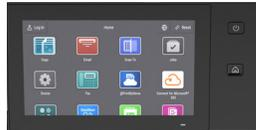
**A customizable, tablet-like touch screen** allows you to do even more in fewer taps and steps. The C625 MFP features a 7-inch user interface (UI) while the C620 has a TBD-inch UI. Both provide easy access to the Xerox App Gallery.
